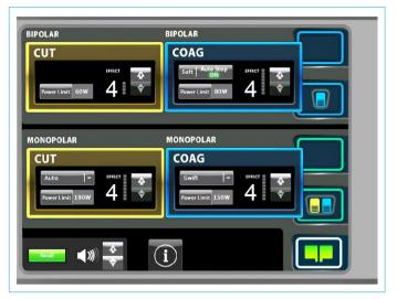
**Figure 3.** Parameters that were set up using The da Vinci Xi<sup>™</sup> robot-assisted surgical system at the time of surgical intervention.
