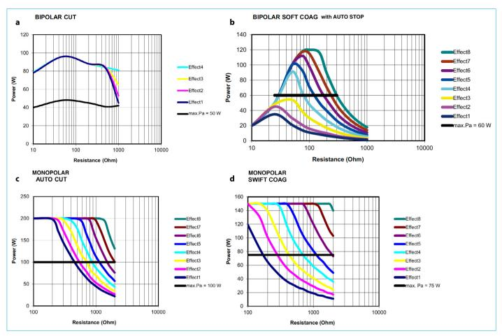
Figure 4. Technical Parameters implicated during the surgery and they were bipolar cut (a); bipolar soft coag with auto stop (b); monopolar auto cut (c); monopolar swift coag (d).
